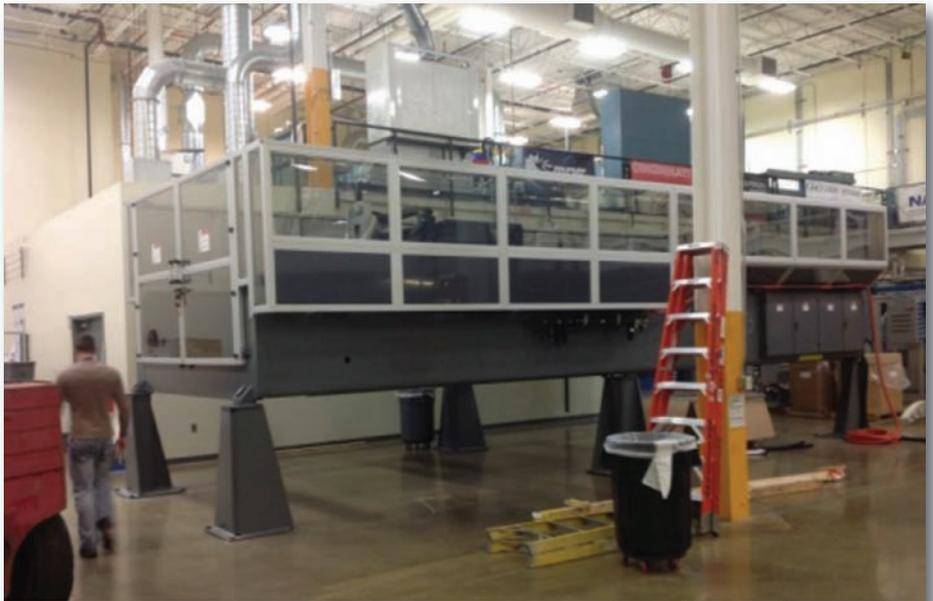
**Figure 6. The largest 3D printer in the world at Oak Ridge National Lab can print metal parts up to 20 feet long**
