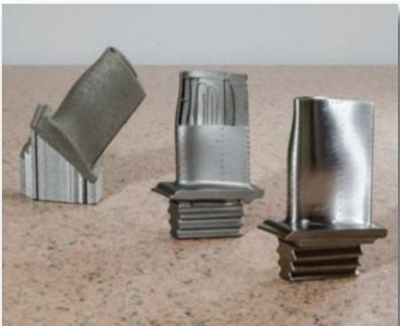
**Figure 5: Turbocam 3D printed these aero-engine turbine blades with intricate cooling channels and complex instrumentation, reducing development time by 80%**
