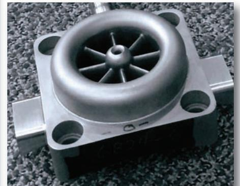
**Figure 2:** This GE fuel injector was produced by 3D printing
